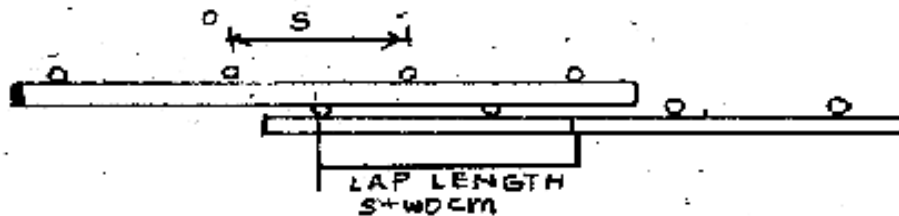
FIG -3 : LAP SPLICING OF WELDED WIRE FABRICS
